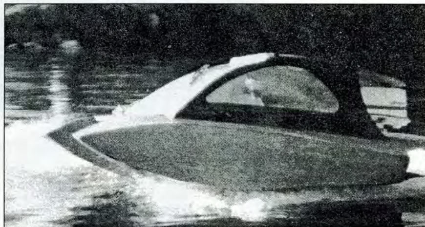
Bill Schmide built this eight-foot plywood boat in 10 days. The Pickle is built in the "tunnel" style from one sheet of plywood.
